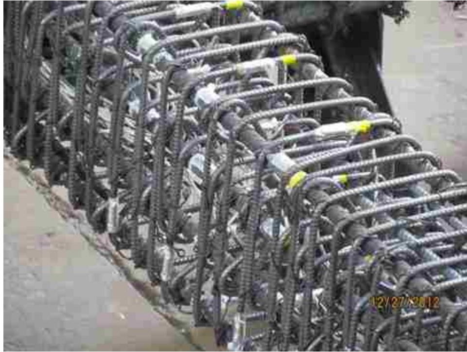
Figure 3-37: Strain gage instrumentation
