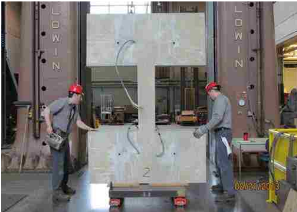
Figure 3-49: Transferring test specimens using rollers
