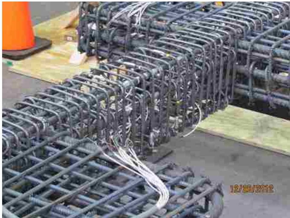
Figure 3-38: Strain gage instrumentation
