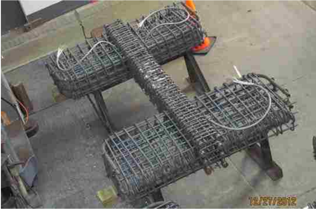
Figure 3-35: Reinforcement of TS01
