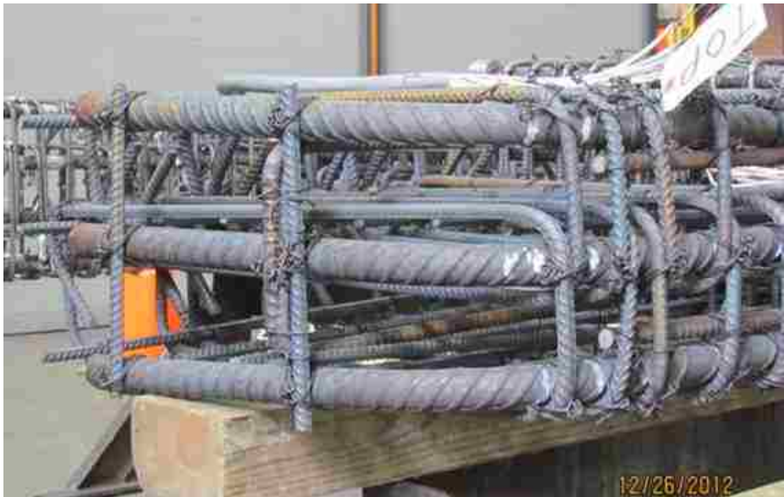
Figure 3-40: 90-degree hook of flexural bars
